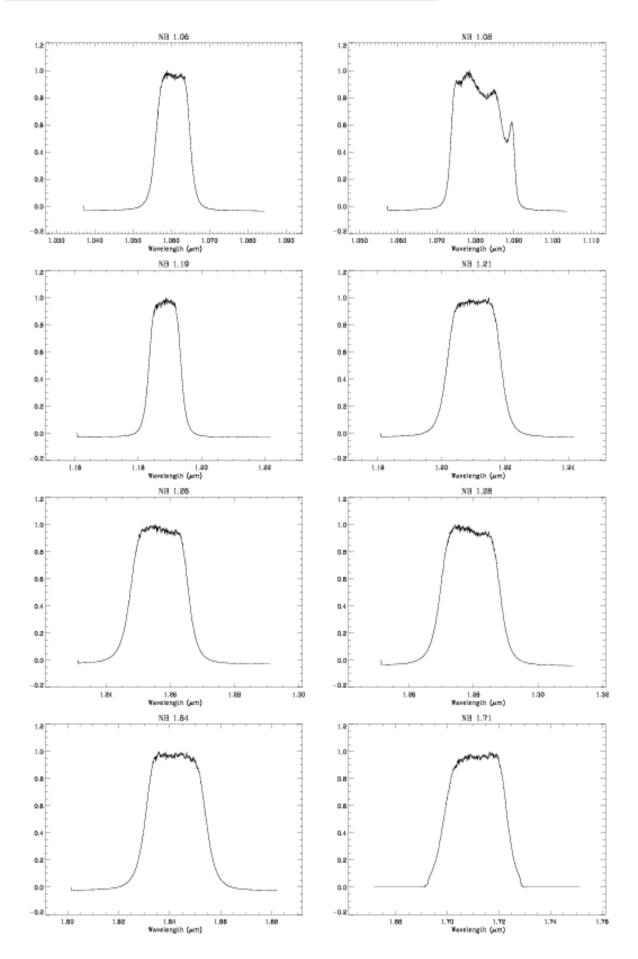
Figure 21: Narrow band filter curves
