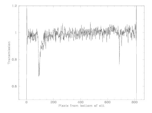
Figure 2: Transmission along 0.8" slit showing two slit defects
