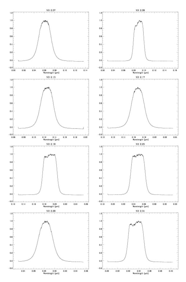
Figure 22: Narrow band filter curves
