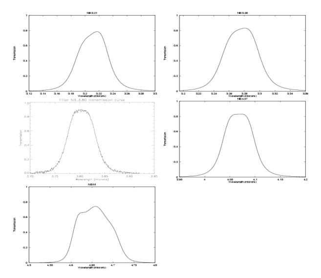
Figure 23: Narrow band filter curves
