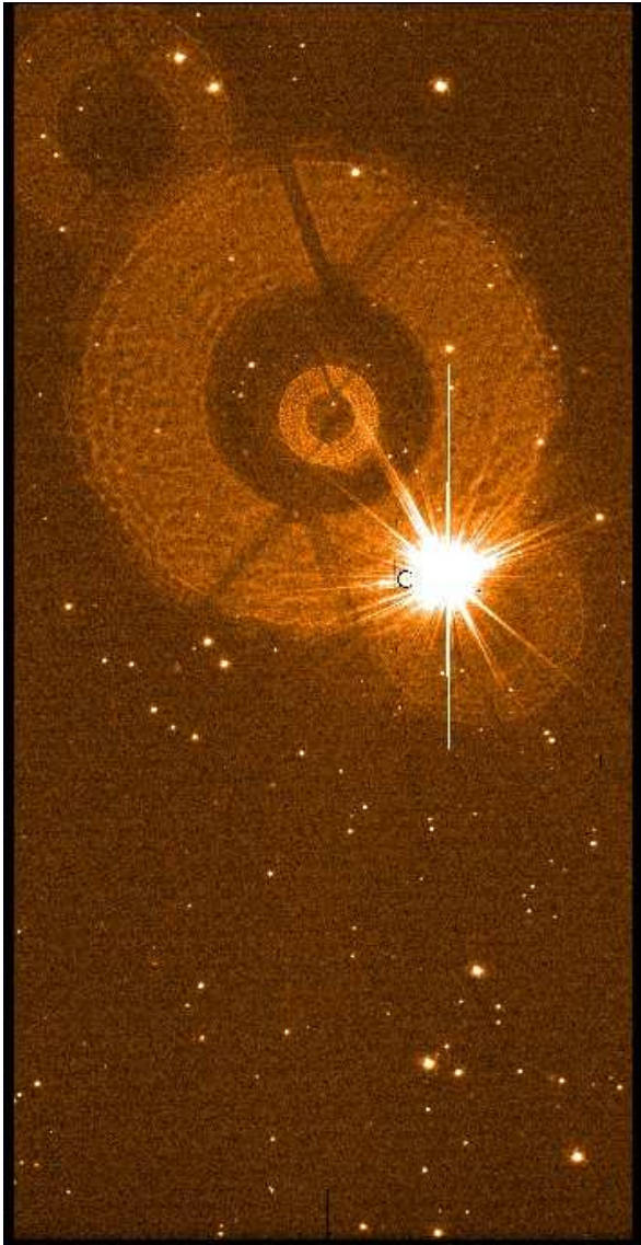
Figure 19: Example ghost reflection from a g' = 6.5 magnitude star in a 60-second g' band exposure, in CCD #91. The ghosts line up along a radius vector through the center of the array, which is towards the bottom right in this case. Appearances will be different in other locations. Ghosts are numbered in order of decreasing surface brightness: from top bottom, numbers 4,2,1,3. The table on the right gives their radii and surface brightness, scaled to a magnitude zero parent star. If stars of this brightness or above as well as OmegaCAM observations were uniformly distributed in the sky, every fourth to fifth field would contain one such star.
