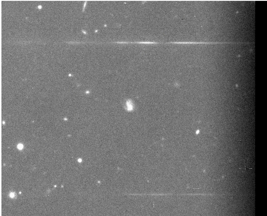
Figure 20: Example of reflection of light from a star (in this case, two stars to the West) outside the field. Such features can occur on each of the four corner CCDs.
