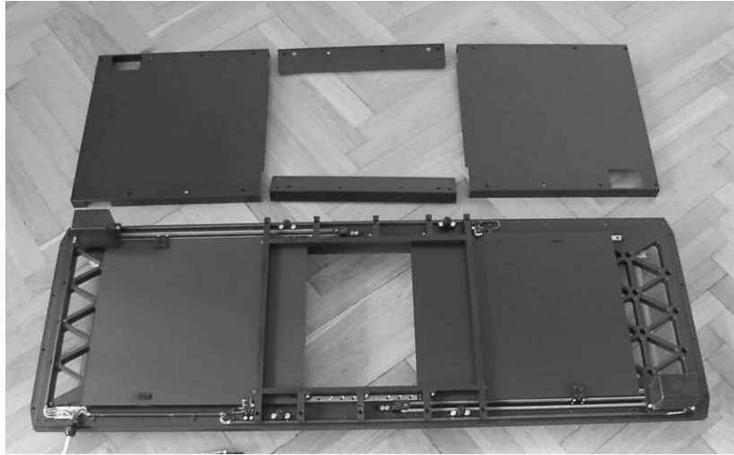
Figure 13: Picture of the partly disassembled shutter unit (Bonn shutter). The two blades, as well as the central aperture, are visible in the lower part of the unit.
