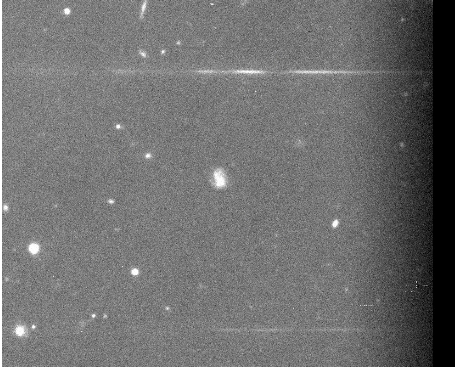
Figure 28: Example of reflection of light from a star (in this case, two stars to the West) outside the field. Such features can occur on each of the four corner CCDs.
