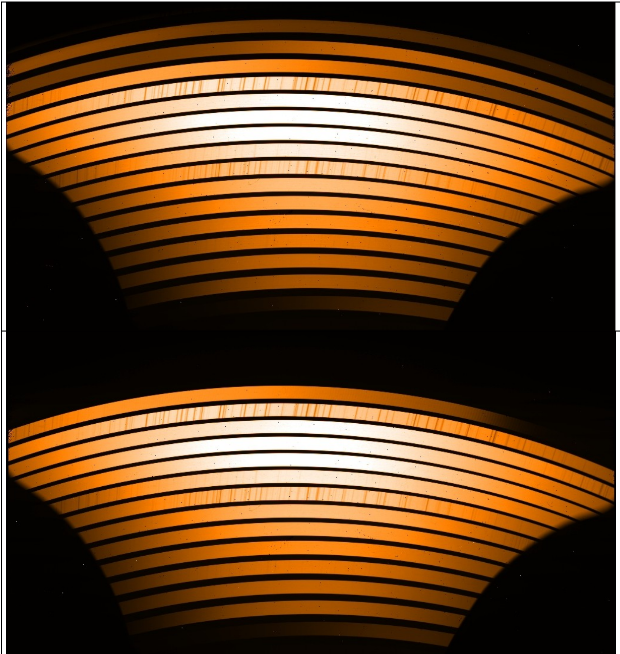
ON-OFF Flat field frames for the normal 0.6" NIR slit (top) and for the 0.6" with blocking filter (bottom). One can easily note that the last orders are cut by the K-band blocking filter.
