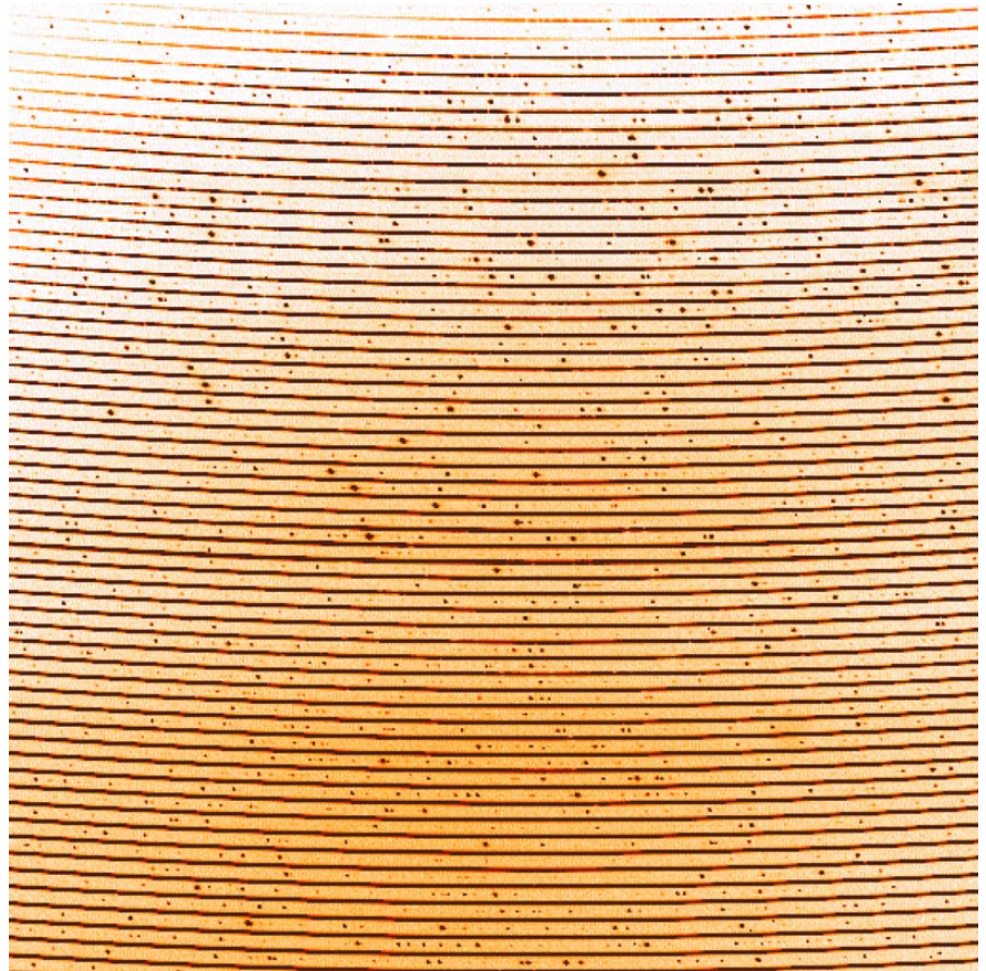
Figure 5: CCD frame of a CORALIE stellar exposure with its simultaneous thorium reference. The emission lines (black dots) of the thorium spectrum are clearly visible between the orders of the stellar spectrum
