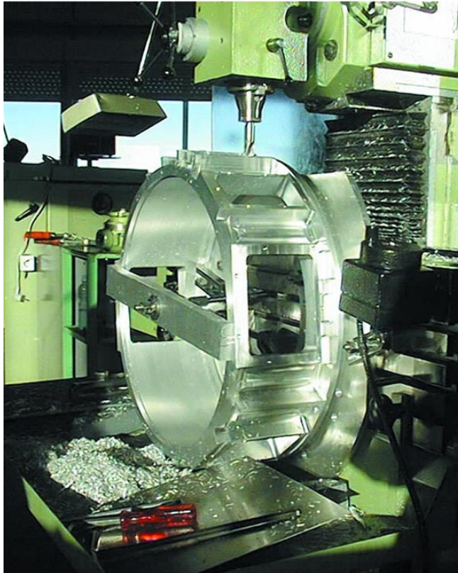
Figure 13: The Cassegrain Fibre Adapter body during manufacturing at La Silla, ESO.
