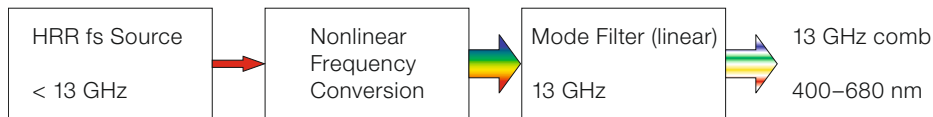
Figure 3 (above): Block diagram for the proposed laboratory demonstrator of the calibration system based on a frequency comb.
