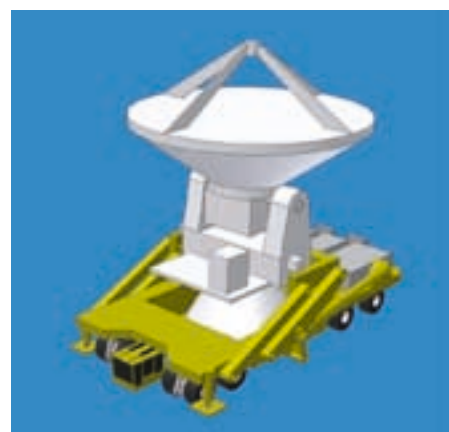
Figure 4. Transporter design with hydrostatically driven wheels.
