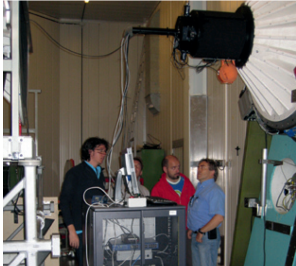
Figure 3. Iqueye at the NTT, with some members of the team and of the supporting staff from La Silla. Two of the four SPADs are clearly seen, protruding from above and below the middle of the instrument. The rack includes the control electronics and the rubidium clock.
