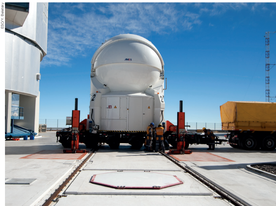
One of the VLTI 1.8-metre Auxiliary Telescopes (ATs) being replaced on its tracks at Cerro Paranal after mirror re-aluminising. Each AT has its own transporter that lifts the telescope and moves it from one observing position to another on tracks. However the transfer by road to and from the coating plant at the base camp relies on a truck, as shown.
