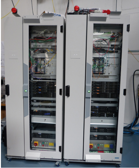
Figure 3. The two SPARTA computers for GRAAL and GALACSI (left). They are based on identical hardware, but run different software codes adapted to the AO modules. These cabinets will be located in the bodega of UT4 to save room on the azimuth and Nasmyth platforms. An optical fibre pair needs
