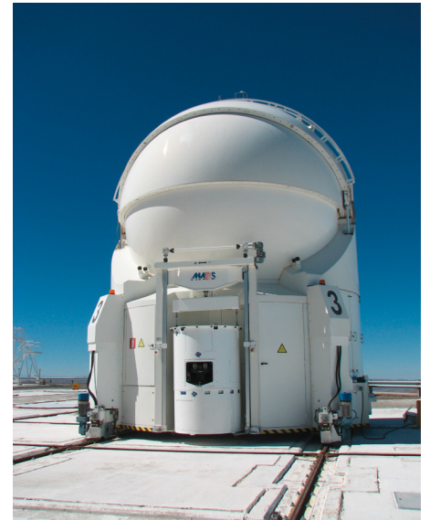
Figure 3. An Auxiliary Telescope with lifted ROS module ready to be moved to a different baseline position.
