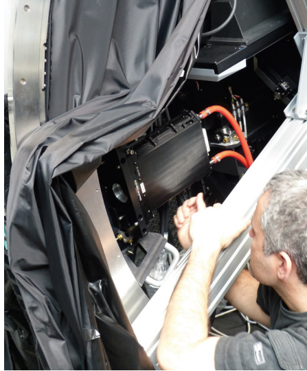
to run to the wavefront sensor cameras for data transfer. A wavefront sensor camera running an e2v L3 CCD CCD220 is shown (right). The camera fulfills the expected performance of < 1 e- readout noise at 1 kHz frame rate.
