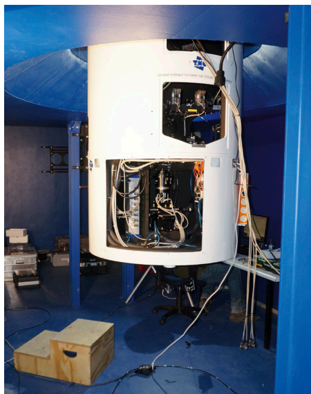
Figure 5. Integration of a new star separator inside the relay optics structure of one of the Auxiliary Telescopes, as seen from the inside of the new maintenance station.
