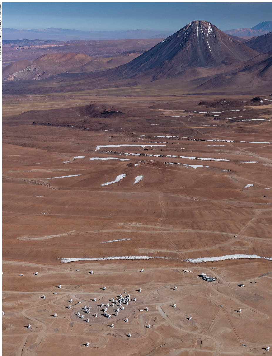
Figure 2. ALMA is located on the Chajnantor Plateau in Chile’s Atacama Desert. At the bottom-center of the image, one can see a set of the fifty-four 12-m antennas. To the left, in the bottom-center, the Atacama Compact Array (ACA) is composed of twelve 7-m antennas and four 12-m antennas. Triangular antenna stations are visible in the image. Each of the 192 available stations can house an antenna, allowing for several array configurations.
