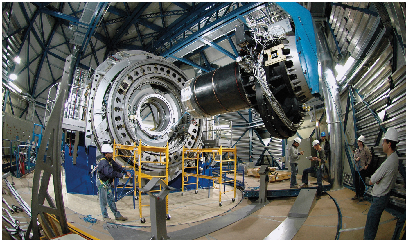
Figure 1. VIRCAM insertion into M1 of VISTA.
