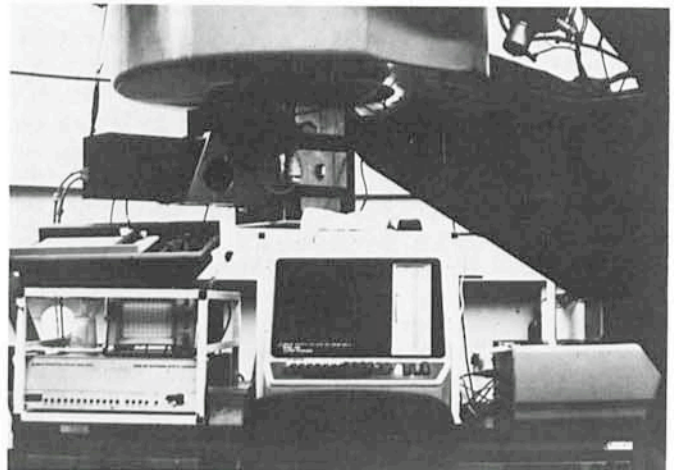
Fig. 2: The area photometer at the 1 m telescope; detector controller, monitor and computer console can be seen in the foreground.
