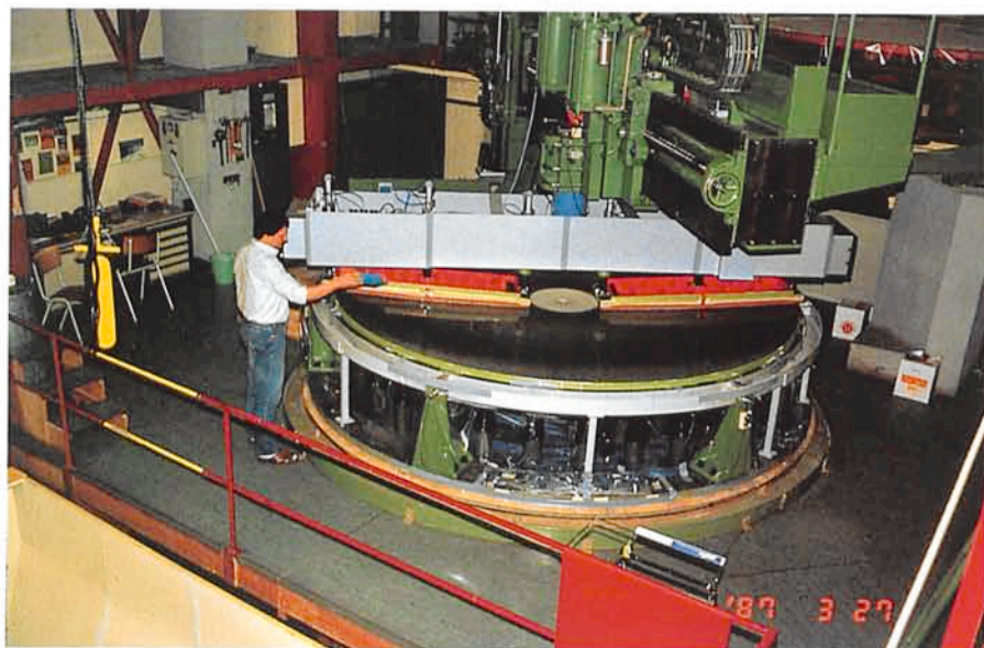
The 3.58-m NTT main mirror being polished at Zeiss, Oberkochen, F.R.G.
