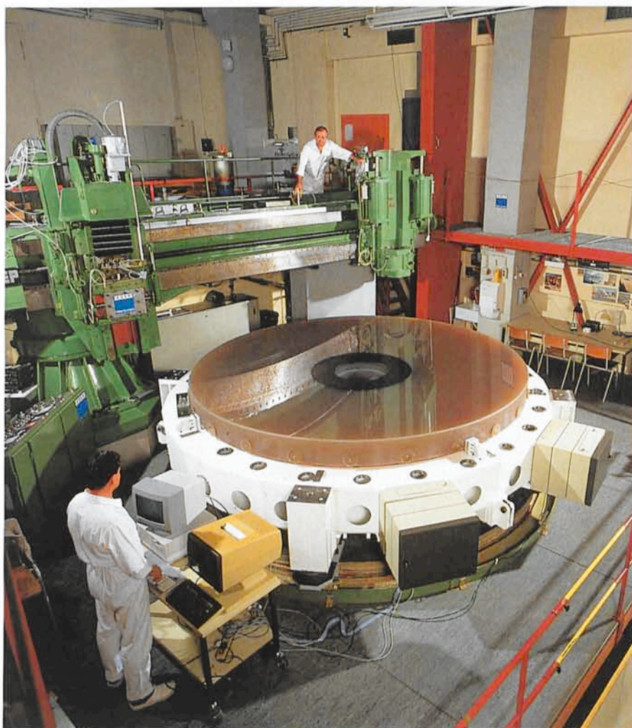
The finished NTT primary mirror at Carl Zeiss in July 1988. The mirror is mounted here on its final NTT support in its cell for testing in the same set-up as was used for manufacture.
