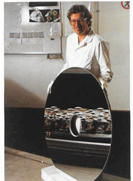
Figure 3: The 1-m test mirror (the thin rim shows the high aspect ratio of 56).
