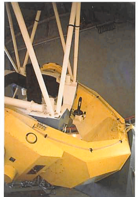
Figure 1: The Differential Image Motion Monitor mounted on the 2.2-m telescope.
