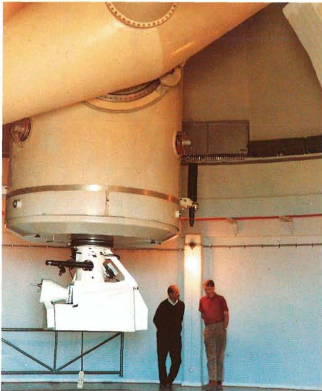
The 1.52-m Telescope equipped with the Cassegrain "Chilicass" spectrograph, borrowed from Marseilles Observatory. In the background, right, ESO's Chief-mechanic Jan Doornenbal talking to an (yet) unidentified person. In the early years, most of the observing time with the spectrograph was devoted to the determination of radial velocities and spectral types of stars in the Magellanic Clouds that had been detected by means of the GPO observations in South Africa.
