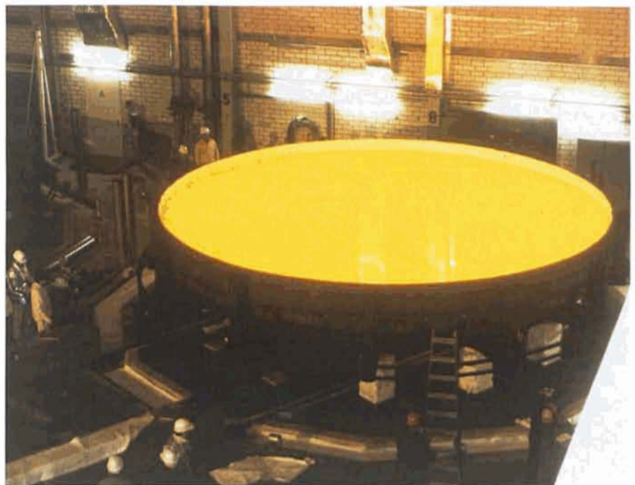
The first 8.6-m mirror blank at Schott, shortly after the molten glass was poured into the rotating form (Photo: Schott).
