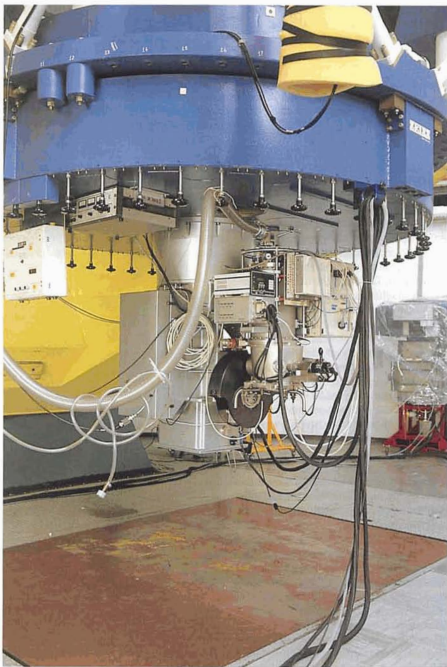
Figure 1: IRAC2 mounted on the F/35 adapter at the 2.2-m telescope.
