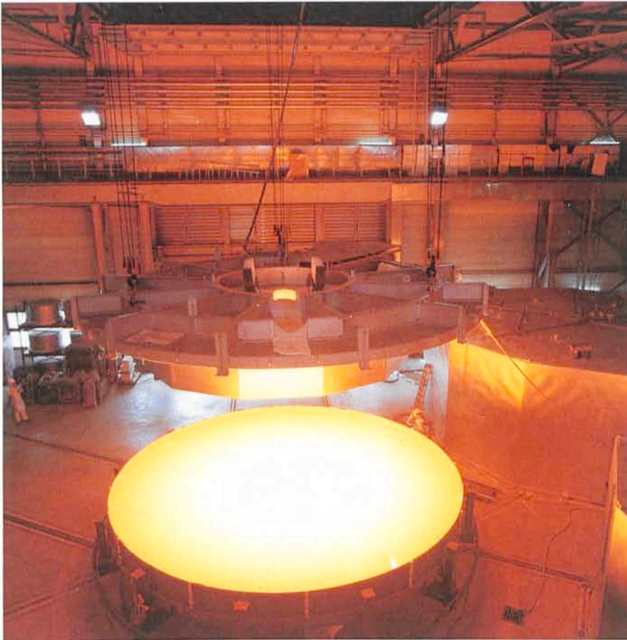
Figure 2: Lifting the overhead heating system.
