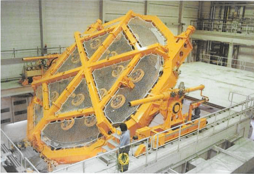
Figure 3: Turning the mirror blank.
