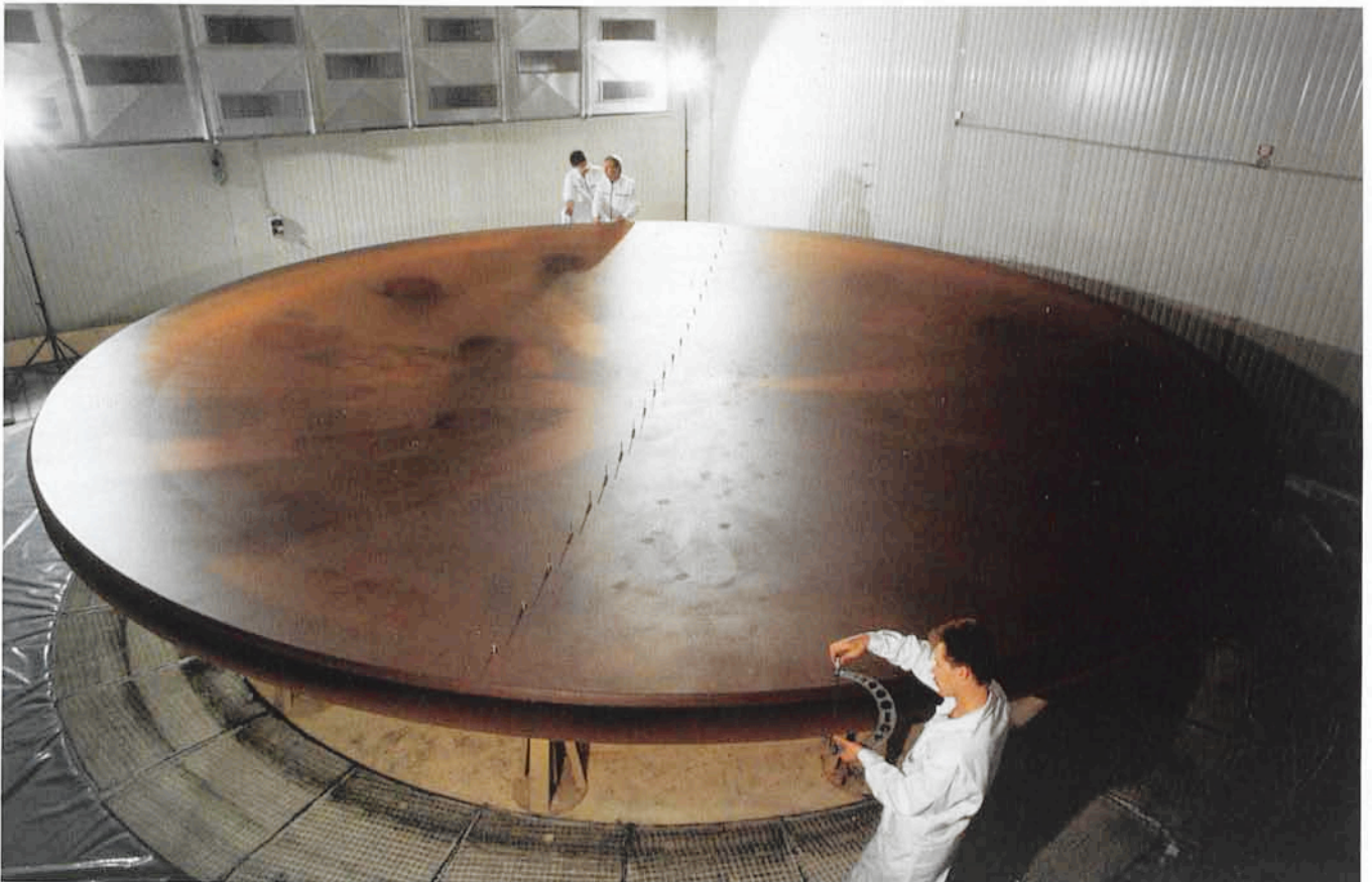
Figure 4: The blank during quality inspection.
