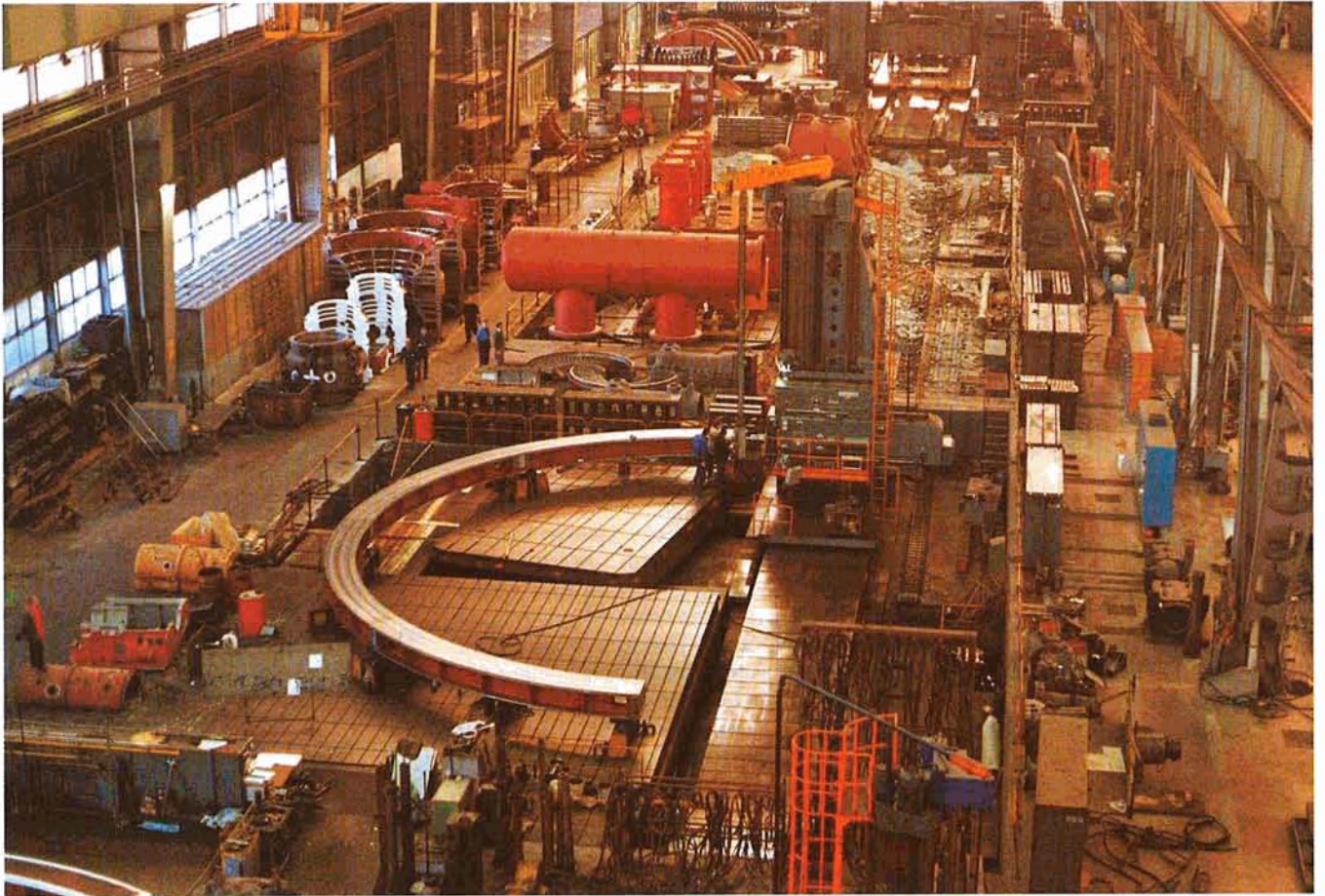
Figure 1: The azimuth outer track segments are laid onto the tooling machine for milling at Ansaldo factory in Genova.
