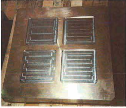
Figure 3: The first series of azimuth axial pads ready to undergo final machining at the factory of Riva Hydroart in Milan.
