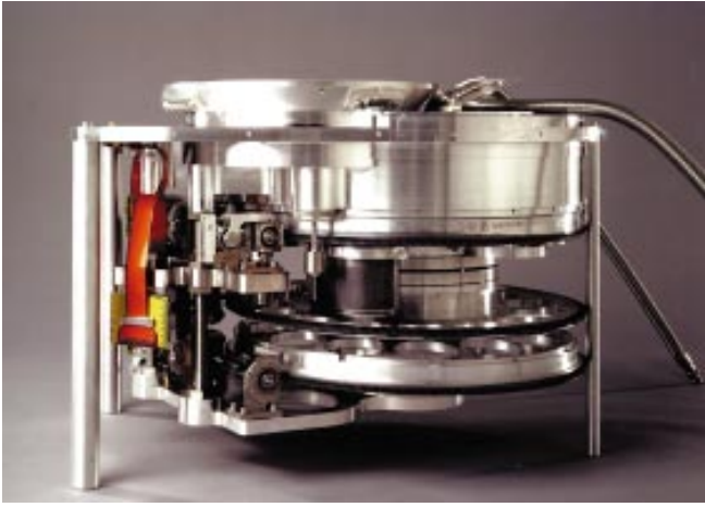
▲ Figure 1: One of the two ISAAC cameras comprising the array detector unit (not shown); the objective wheel and two filter wheels. In common with most moving functions, the wheels are driven by 5-phase stepper motors and spring loaded worm gears acting on the large toothed rings.
