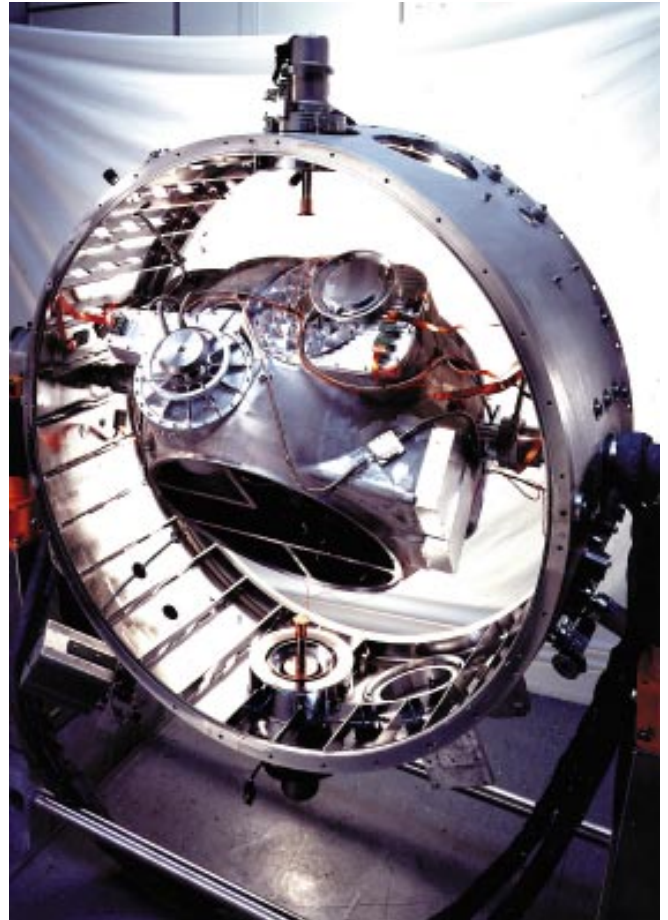
Figure 2: The partly assembled instrument showing the cryogenic optical assembly with one of the cameras mounted (only the detector unit visible at the top right) provisionally supported in the vacuum vessel.
