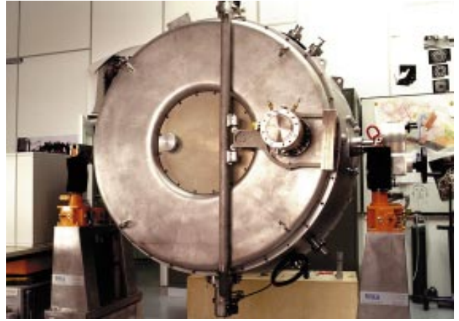
▲ Figure 4: Rear view of ISAAC fully integrated in its vacuum vessel. The closed-cycle coolers at the top and bottom are mounted on bellows and connected by the long bar to minimise vibrations. Also visible to the right is the permanently mounted magnetic bearing turbomolecular pump used to evacuate the vessel.
