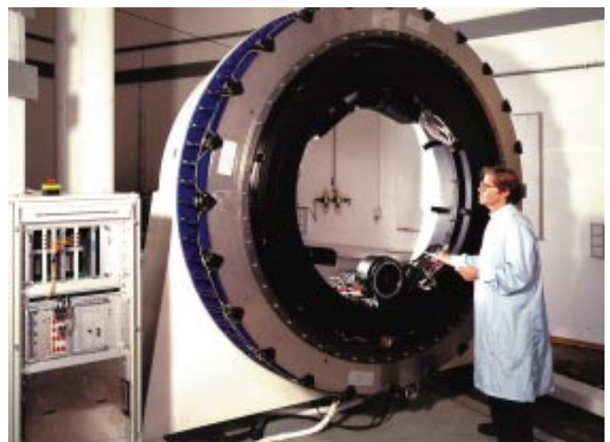
Figure 6 shows the first of the 12 adapter/rotators in the Garching assembly hall during integration and testing. The Beryllium arm that will explore the focal plane has not yet been integrated. On the left-hand side, one can see the electronic test rack used to collect all parameters for final analysis and performance of the machine.
