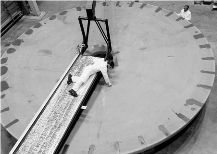
Figure 4: Preparation for the measurement of residual stresses (birefringence measurements).
