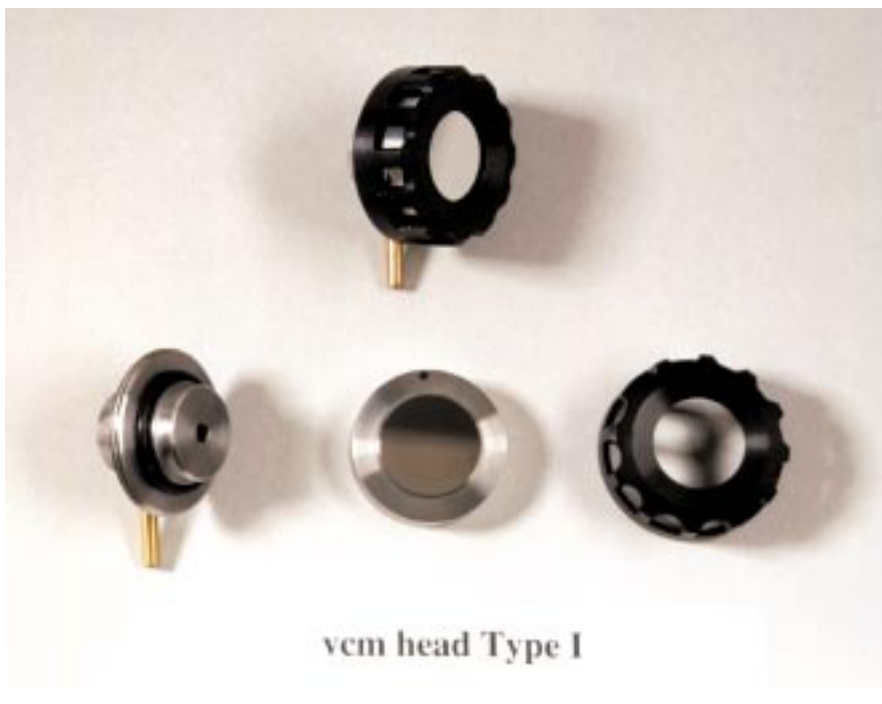
Figure 1: Variable Curvature Mirror mounted and unmounted with its support. The active part is a very thin (300mm) meniscus and the deformation is achieved with a uniform air pressure applied to the back side of the mirror. The optical aperture is 16 mm.
