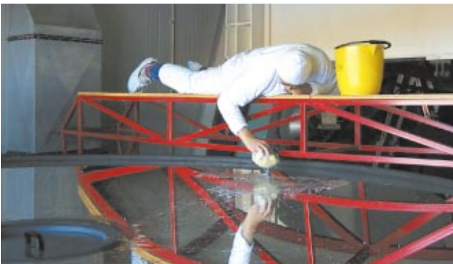
Figure 1: Alain Gilliotte, optician engineer at La Silla, is starting to wash the NTT main mirror, with a solution of soap and water and a sponge.
