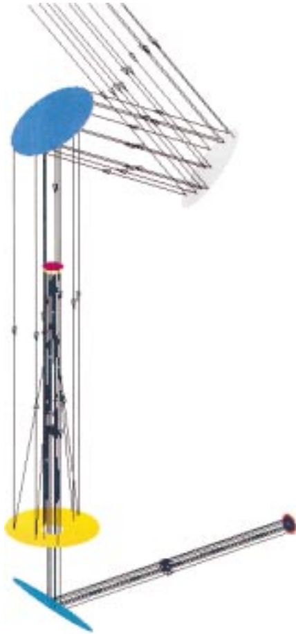
Figure 1: Three-dimensional representation of the VLTI Test-Siderostat Optical Path. The diameter of the Siderostat mirror is 400 mm and the second plane mirror (upper part of the periscope) is at 25° angle of elevation. The use of a Beam Compressor allows to have an 80-mm output pupil (similar to the ones of the Unit Telescopes).
