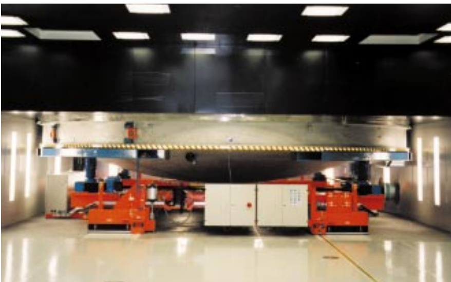
Figure 2: The lower part of the coating unit vacuum chamber. For loading and unloading of the mirrors, the lower half of the chamber is moved on 8 air-cushions from the coating unit location to the mirror handling tool and vice versa.
