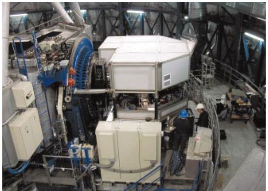
Figure 3: UVES. When the UVES cover is put in place, it protects the sensitive inner parts of the instrument from unwanted light and dust. (This digital photo was obtained on September 16, 1999.)
