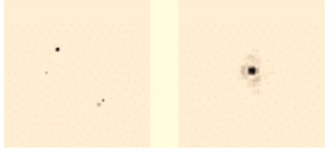
Figure 1 Left: simulated multiple-point source truth (4 sources). Note that each star is centred on a single pixel. Right: sample PSF from the data cube. Note the diffraction-limited core and Airy rings broken up by residual aberrations. (Both images displayed on a square root scale.)
