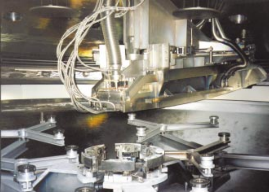
Figure 3: A look into the coating unit vacuum chamber. The upper vacuum chamber part carries the DC planar magnetron sputter source. In the lower part the rotatable whiffle tree for support of the primary mirror is visible.
